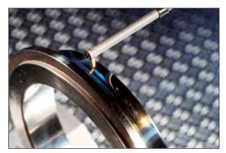
measureable form features may be spherical, aspherical, concave, convex, internal or external
