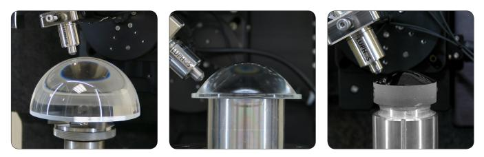
LuphoScan platforms are scanning interferometers based on an optical (non-contact) point probe that utilizes MWLI<sup>®</sup> technology (multi-wavelength interferometry).
