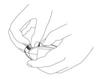
To remove the batteries from the Traverse Unit, remove the battery cover and then press down on the edge of the battery closest to the centre-line of the Unit. The top battery can then be slid out of the battery compartment. The remaining batteries can be removed by tipping them out of the Unit. Replace the battery cover.
