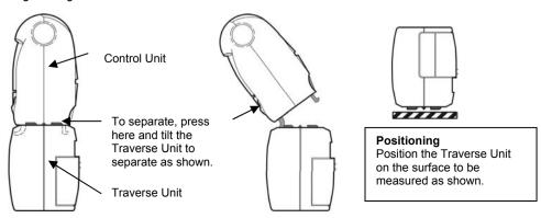
To return the unit to its storage configuration, reverse the above procedure.
