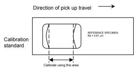
On the Control Unit press the Mode Select buttons until  $\sqrt{}$  is indicated on the Mode status. Press the Start button on the Control Unit. This will initiate the gauge calibration procedure. At the end of the calibration procedure the Control Unit will display the results of the calibration. The Ra value should be 5.81µm and the Rz value 21.5µm. If an error occurs an E code is displayed.
