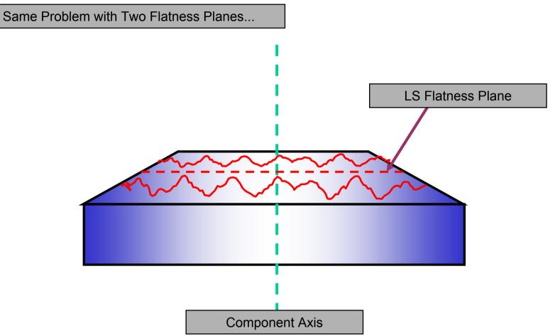
Even if the operator chooses to measure using multiplane flatness the results will still show good squareness. This is because if more than one flatness planes is measured then an average plane is fitted to all measured data, the result will again indicate good squareness.
