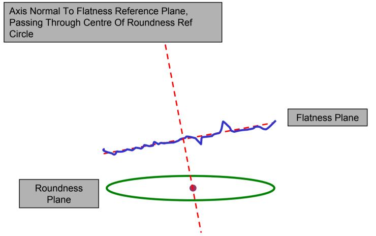
The above diagram shows the description of a roundness/flatness axis generated from a single roundness and flatness measurement.
