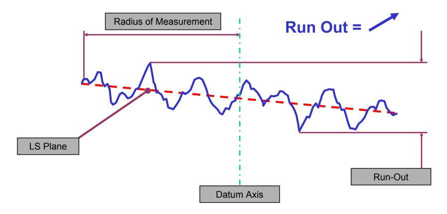
Run-out is the minimum separation of two axial planes normal to the datum axis which totally enclose the profile.
