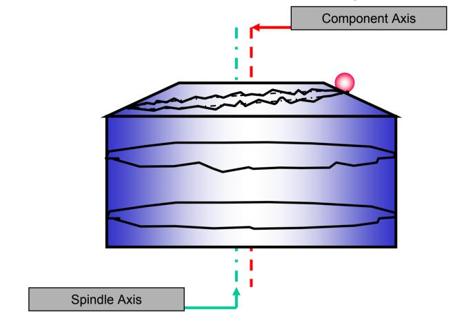
In this diagram we can see that two roundness measurements have been made in order to construct an axis. A flatness measurement is then made in order to assess squareness to the created axis.
