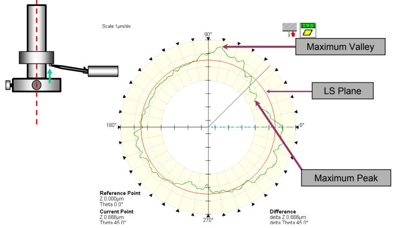
Now when we analyse flatness because the surface is upside down (stylus contact direction up) then deviations on the outside of the LS plane are valleys and deviations on the inside of the plane are peaks.
