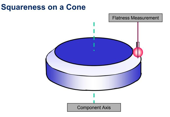
Although it is possible to measure the flatness of a cone along a single trace, squareness is not possible. In this example an axis is constructed through the base of the component and saved as a datum. A flatness measurement is now made around the conical area of the part.
