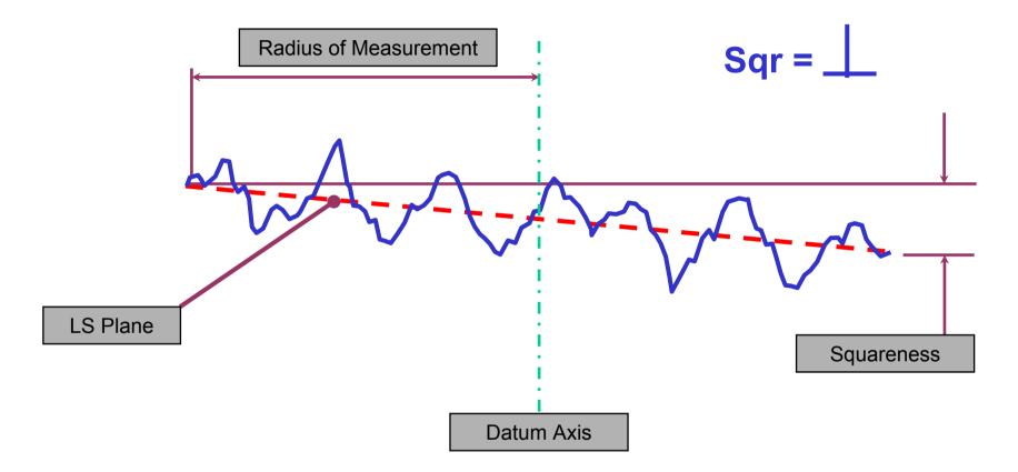
The squareness value is the minimum separation of two parallel planes normal to the reference axis that totally enclose the reference plane.
