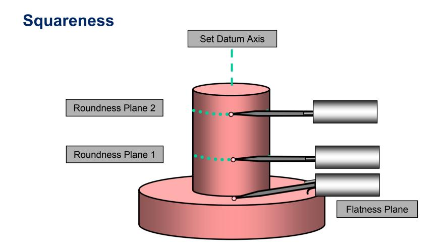
The above slide shows the method of analysing the squareness of a flatness plane with respect to a pre defined datum axis, in this case an axis created from two roundness planes.
