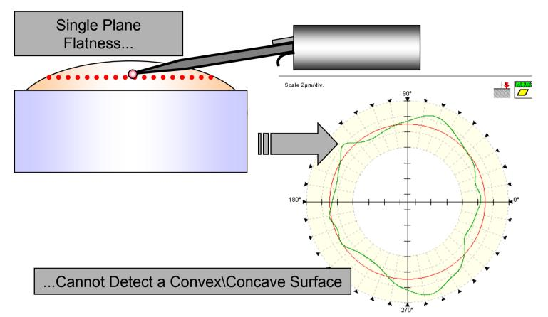
A single plane flatness measurement is usually sufficient on most components. However, a single flatness plane will not be able to show if the component surface has a convex or concave form.
