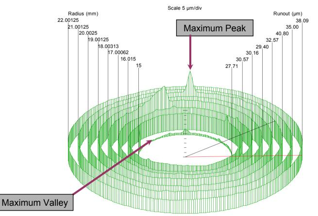
On a lot of flatness measuring systems it is possible to combine the results of a flatness measurements. In the case above 7 flatness planes have been measured, the overall flatness is calculated by fitting a Least squares or Minimum zone flatness plane through all of the data.
